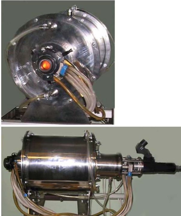
Fig. 1 Photographs of the furnace
